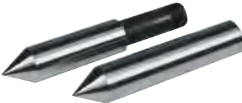
Centring points 004-57 60° carbide tipped Shank of centring points: dia. 16 mm
