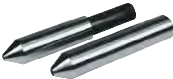
Centring points – hollow centres 004-56 with centring hole DIN 332-A1, 6 x 3.8
