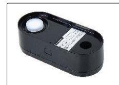
white and black calibration cavity (included)
