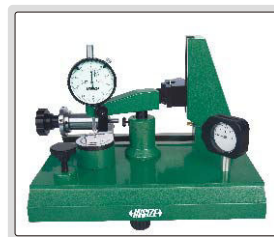
check the effect of lateral force on accuracy of dial indicators (half round gage block is required)
