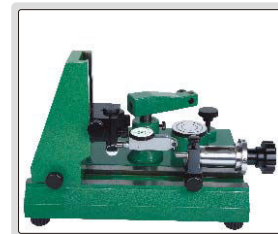
inspect accuracy of test indicators
