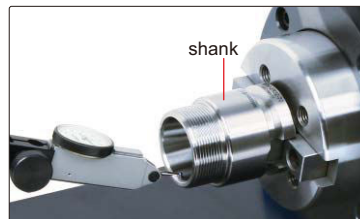
measure radial runout of shank
