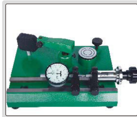
inspect accuracy of dial indicators (range 0-25mm)
