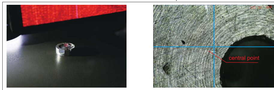
laser indicator locates the central point
