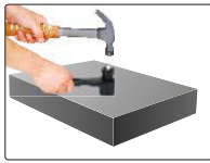
hammer impact to apply test force
