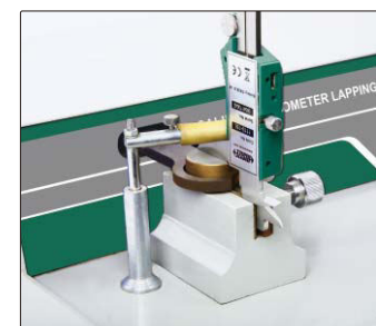
lapping measuring surfaces of caliper lower jaws
