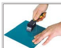
step 1: make grid cutting on surface
