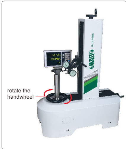
rotate the handwheel to rotate tools
