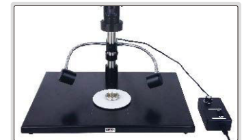
illumination direction and brightness are adjustable
