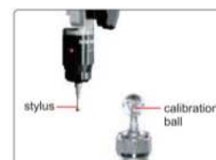
probe (optional), includes Ø2mm and Ø3mm styli, Ø25mm calibration ball, measuring accuracy is 10μm
