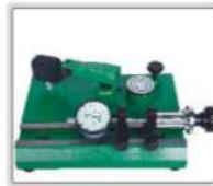
inspect accuracy of dial indicators (range 0-25mm)
