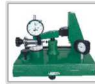
test the effect of lateral force on accuracy of dial indicators (half round gage block is required)
