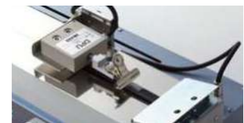
Peel test of embossed carrier tape
