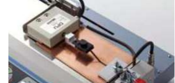
Peel test of copper foil
