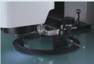
Sonda TP20 s opti-fix upinkami
