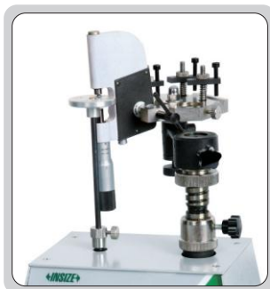
check the measuring force of indicating micrometers
