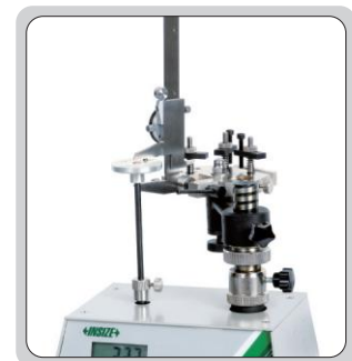
check the measuring force of calipers
