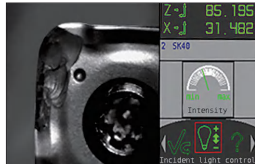
check cutting edge wear
