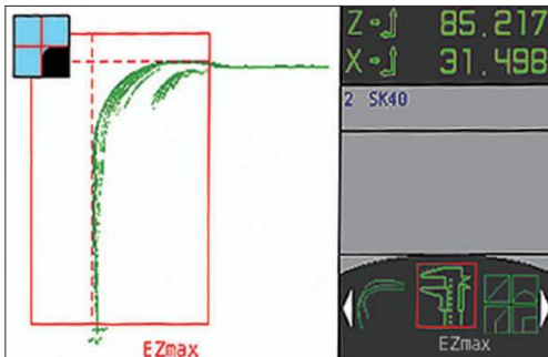
scan and measure the maximum profile of the cutting tool
