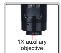
1X auxiliary objective (included)
