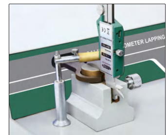
lapping measuring surfaces of caliper lower jaws
