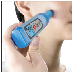
pH "plane type" electrode (optional)
