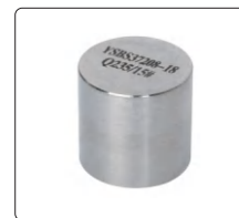
15# steel control sample (optional)
