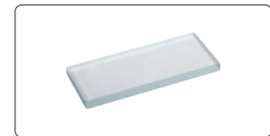
50mm reading scale (check magnification accuracy)
