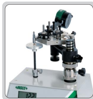
check the measuring force of bore gauges
