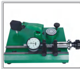
inspect accuracy of dial indicators (range 0-25mm)
