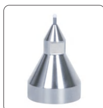
3mm zircon ball probe (included)
