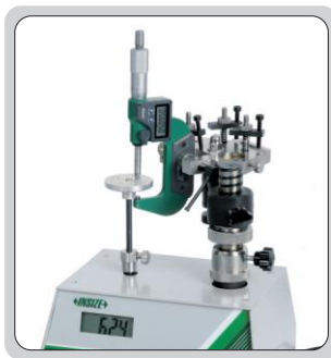
check the measuring force of micrometers
