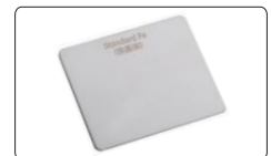
Fe zero calibration plate (included)
