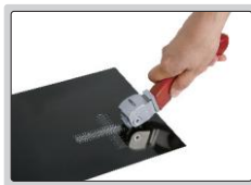
step 1: make grid cutting on surface
