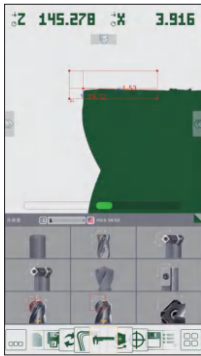
fast measurement, automatic recognition of cutting edge shapes
