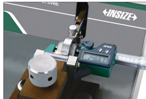
lapping measuring surfaces of outside micrometer
