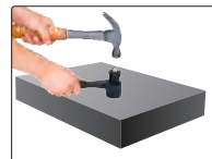
hammer impact to apply test force
