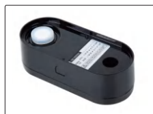
white and black calibration cavity (included)
