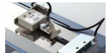
Peel test of embossed carrier tape
