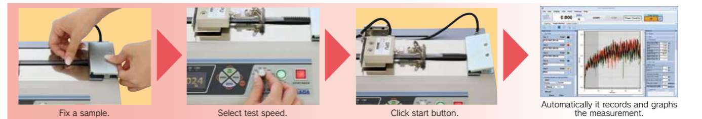
Peel test of copper foil
