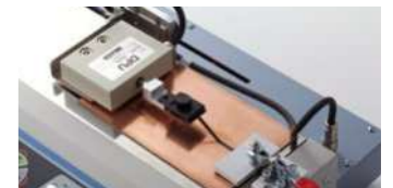
Peel test of copper foil
