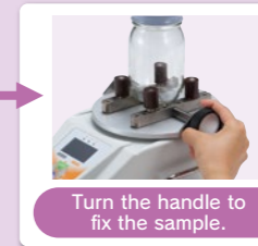
Put pins in holes with consideration for sample's size.
