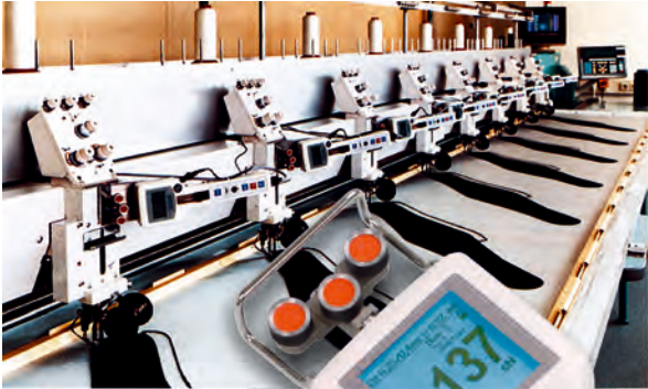
In the Aircraft Industry producing parts made by fiber-reinforced materials for airplanes on embroidery machines
