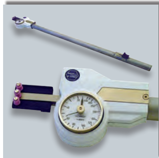
Model DX2 With extension handle and ceramic pins to reach critical measuring positions
