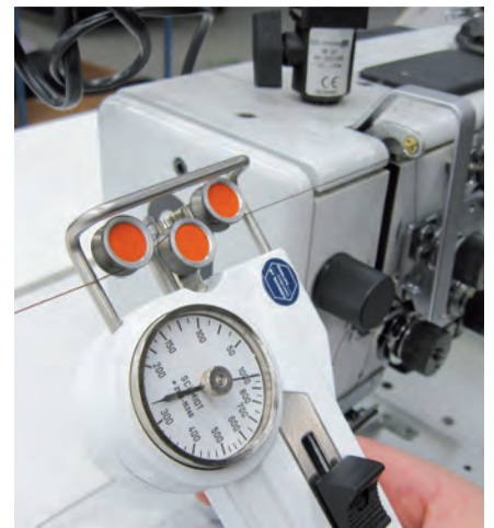
In the Sewing Industry For adjusting yarn break on industrial sewing machines e. g. production of airbags
