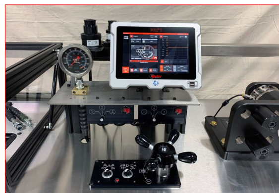
T-Box™ 2 at the center of a test bench for manual torque wrenches, powered torque tools and hydraulic torque wrenches
